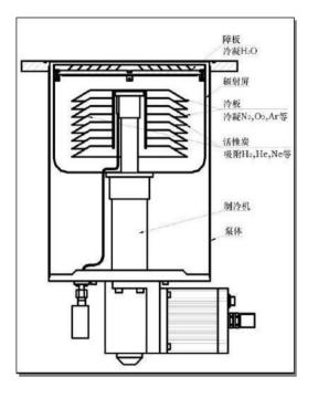
Cryogenic pump is also called low temperature vacuum pump, cold pump, condensate pump. The cold source of the cryogenic pump can be cryogenic liquid (liquid nitrogen or liquid helium), or it can be a cryogenic refrigerator. The cryogenic pump is introduced here. The cryogenic pump's cryogenic machine generates refrigeration at two temperature stages, respectively cooling two cryogenic surfaces, on which the pumped gas is cooled.
